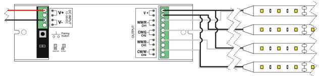
Multiple different colors of strips may also be connected in the same way as single color strips, but will adjust simultaneosly and will not be able to be dimmed indpendently.
