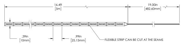
Strip thickness is 0.06in. (1.52mm)
