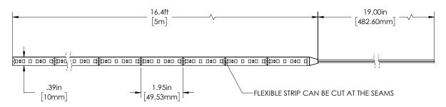
Strip thickness is 0.06in. (1.52mm)
