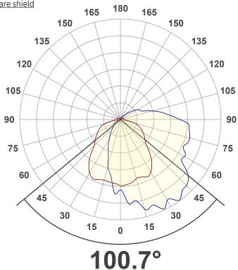
Beam angle is representative of all WPG models. Additional model-specific photometric data available on site or upon request.
