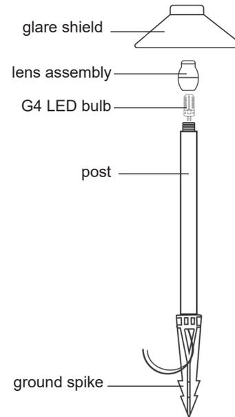
Note: Assemble fixtures as shown. Run wires through slot in stakes.
