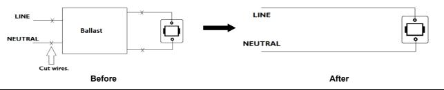
The 2-pin diagonal and 4-pin sockets have different wiring configuration.
