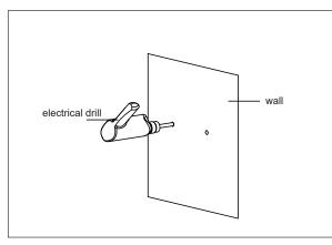
1. Use the mounting bracket to mark out bolt holes on the wall and then drill holes.(Fig 1)
