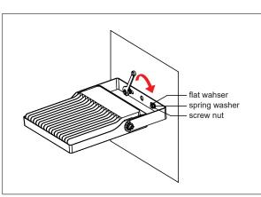
2. Drive the bolts into the holes with the
