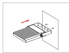
3. Place the mounting bracket over the bolts and push it flush with the wall.(Fig 3)
