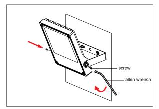
5. Rotate the light to the desired angle and tighten screws with an allen driver. (Fig 5)
