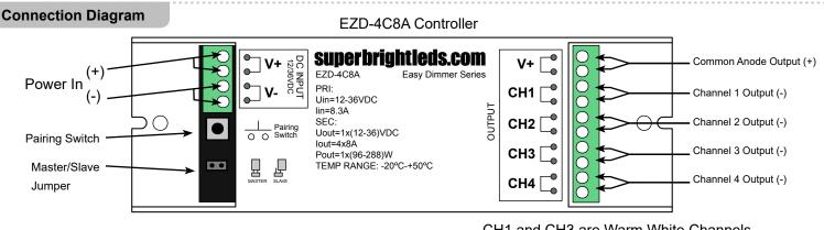
CH1 and CH3 are Warm White Channels CH2 and CH4 are Cool White Channels
