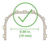
Bends less than 15mm will damage circuit traces and void warranty. Bending strips at sharp angles will damage circuit traces and void warranty.
