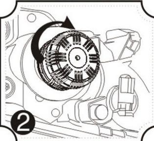
**2** Rotate clockwise to lock in place.
