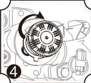
**4** Gently rotate light clockwise until locked in place.
