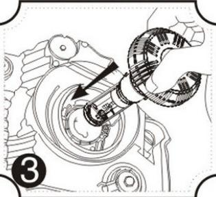
**3** Line up and install light into mounting flange.
