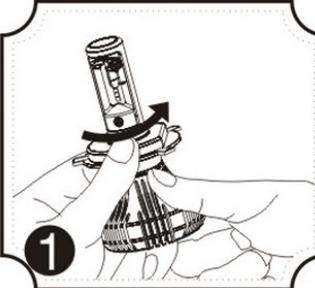
**1** Turn mounting flange counterclockwise to release bayonet-style connection and remove flange.
