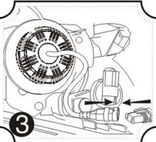
**3** Connect light to vehicle wiring harness.
