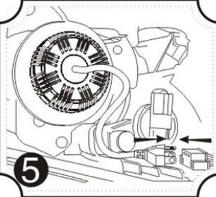
**5** Connect light to vehicle wiring harness.
