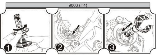
Turn mounting flange counterclockwise to release bayonet-style connection and remove flange.
