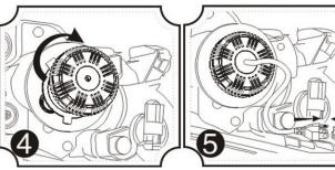
Gently rotate light clockwise until locked in place.
