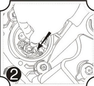
**2** Install mounting flange into headlight housing.
