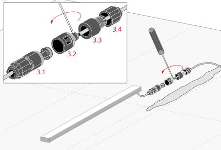
Detach the items (3.2; 3.3; 3.4) of the hermetic coupler from item (3.1). Lead the cable (2) through them and screw it to the socket in item (3.2).
