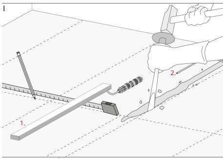
Prepare the groove in the floor for the cable (2).
