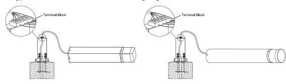
2. Rotate bollard and place in position over bollard base.
