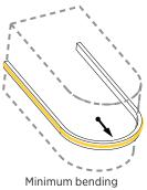
Minimum bending radius ≥ 1.1 in [30 mm]
