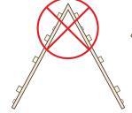
Bending strips on horizontal plane will damage circuit traces and void warranty.
