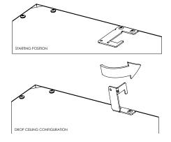
4. Lay fixture into T-grid.
