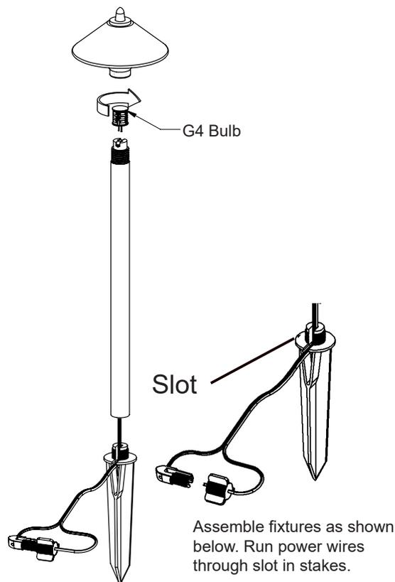
Assemble fixtures as shown below. Run power wires through slot in stakes.
